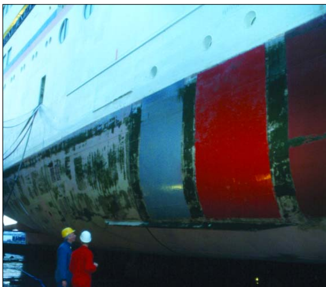
Figure 7.2 After an 11-month worldwide cruise, biocide-free patches on the cruise liner Columbus (Hapag Lloyd Kreuzfahrten) proved more efficient against fouling than the copper-based paint on the rest of the hull. Columbus is one of 19 vessels taking part in a multi-stakeholder project initiated and coordinated by the World Wide Fund for Nature (WWF 2001).
